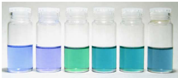
Figure 2. Color changes of ligands in \text{CH}_2\text{Cl}_2 in the presence of anions (3 equiv of TBA salts). From the left: 4 ; 4 + \text{H}_2\text{PO}_4^- ; 5 ; 5 + \text{Cl}^- ; 5 + \text{H}_2\text{PO}_4^- ; 5 + \text{F}^- .
